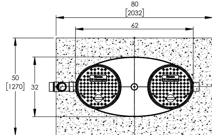
ANCHORING SLAB DETAIL
