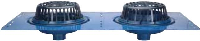
If code requires a primary drain and an overflow drain side by side, the Z163 (shown above) is an ideal solution. It can provide spacing to grid around the drains and easy installation with the Zurn Top-Set™ deck plate. The Z163 can also be incorporated with drain risers (-DR option) which allows for easy vertical adjustment.
