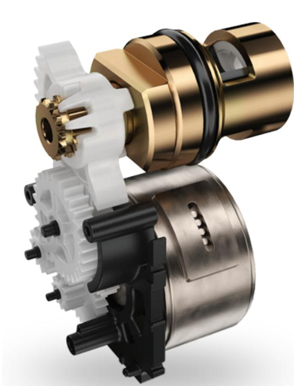
The ceramic disc cartridges wipe against each other in a way that self-cleans and prevents debris buildup. TPE-constructed components, such as the diaphragm, gaskets, and seals, resist corrosion. The combination of these attributes and components allows motor-gear solutions to tack on more years to their lifespan—typically lasting around one million cycles more than solenoid operated solutions.
