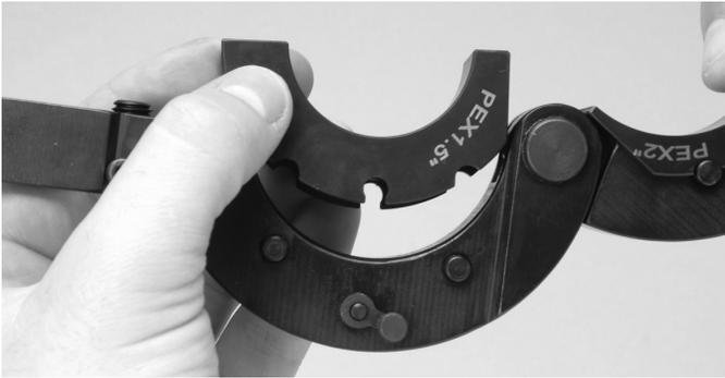
**Step 4:** Rotate key back into position until key clicks to lock jaw in place. Repeat for other jaw.
