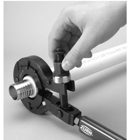
**Step 5:** Drive the nut down with an impact wrench until blue LED light turns on.
