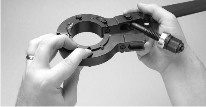
**Step 2:** Continue to hold in the keyed slot, turn tool around and move key out of position. Remove jaw from clamp.
