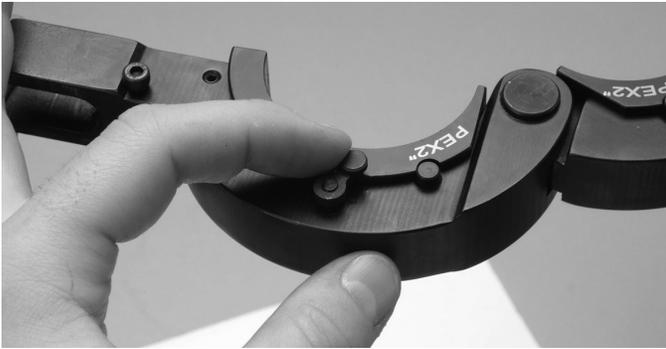
**Step 3:** Insert new crimping jaw.
