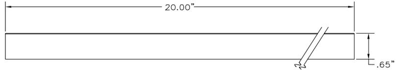
**Engineering Specification:** Provides enhanced heat transfer from Zurn PEX® tubing to underside of wood subfloor. Leave 3" to 6" between plates.
