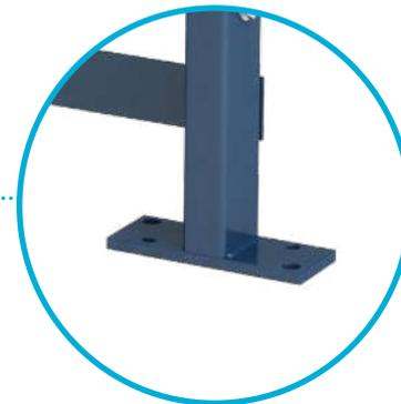
Offset diagonal bolt pattern allows for two 3/8" or two 1/2" anchors per leg
