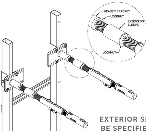
EXTERIOR SLEEVE EXTENSIONS CAN BE SPECIFIED FOR BEHIND-STUD OR BLOCK-WALL APPLICATIONS
