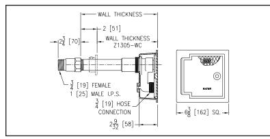
**ENGINEERING SPECIFICATION:** ZURN Z1305 Encased, non-freeze, flush wall hydrant with bronze casing, all bronze interior parts, non-turning operating rod with free-floating compression closure valve, replaceable bronze seat and seat washer, and combination 3/4" [19 mm] female or 1" [25 mm] male straight IP inlet. Nickel bronze box and hinged cover with operating key lock and "WATER" cast on cover.
