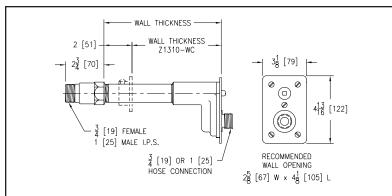
**ENGINEERING SPECIFICATION:** ZURN Z1310 Exposed Ecolotrol anti-siphon automatic draining wall hydrant. Complete with non-freeze integral backflow preventer, bronze casing, all bronze interior parts, non-turning operating rod with free-floating compression closure valve, replaceable bronze seat and seat washer, and combination 3/4" [19 mm] female or 1" [25 mm] male straight IP inlet. Stainless steel face with operating key.
