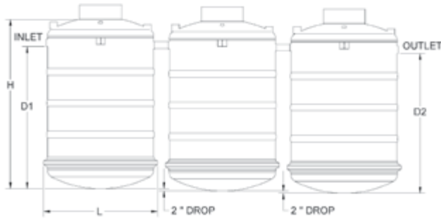
System 3 : Three Tanks in Series
