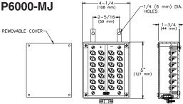
ENGINEERING SPECIFICATION: Zurn P6000-MJ - The Mini Junction Box is a 4-1/4" [108mm] x 5" [127mm] x 1-3/4" [44mm] electrical enclosure designed to connect up to ten Zurn sensor unrinals/closets. The unit includes a high impact plastic enclosure with polarity marked terminal board, high impact plastic cover panel, wall mounting tabs, integral strain relief, and illustrative wiring diagram.
