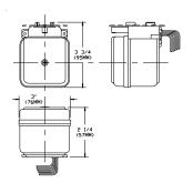
**ENGINEERING SPECIFICATION: Zurn P6000-BB AquaSense** Battery Backup - The battery backup module is designed to supply power for up to 10 ZEMS - sensor flush valves in the event of main power failure. The battery backup is furnished complete with battery pack, mounting plate for battery pack, low battery indicator light, mounting plate for indicator light and batteries (4 "D" cell alkaline batteries).
