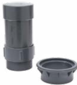
-CE EZ-SET™ Coupling (Patent Pending) with Integral Test Cap Cut coupling flush with finished wall following pressure testing, without removal, reducing installation time (5" min.)
