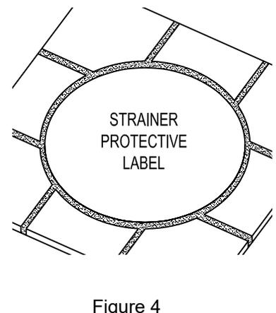
8. Remove backing from strainer label and place onto strainer/frame, ensuring the label is not overhanging the frame edge.
