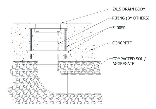
Attach threaded rods of Z400SR to underside threaded bosses of the drain body. Feed rods through the (4) holes of the Z400SR plate and hand tighten set screws at desired length. Attach drain body and Z400SR assembly to pipe stub and tighten set screws against pipe. Adjust threaded rods and set screws until drain is firmly attached to pipe and level. Pour structural slab to top surface of drain body.
