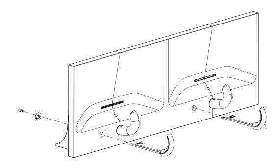
For ease of installion, lay basin on its back. Install the soap spout on right or left soap hole as applicable. Refer to soap dispenser installation guide for details.
