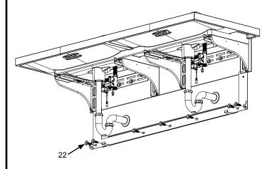
• Re-install wall bracket with coarse screws in previous location. Then, fasten the wall bracket with 3/8" bolts through each holes and into the toggle bolts.
