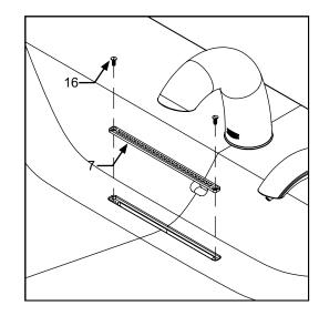
Use T10 Torx wrench to attach the grid drain to basin. Torque screws until the screw heads are flushed with the screw pocket of grid drain.
