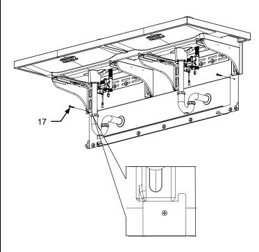
Align wall bracket as shown and install coarse screw on each side. Mark the slots in the wall bracket on the wall.
