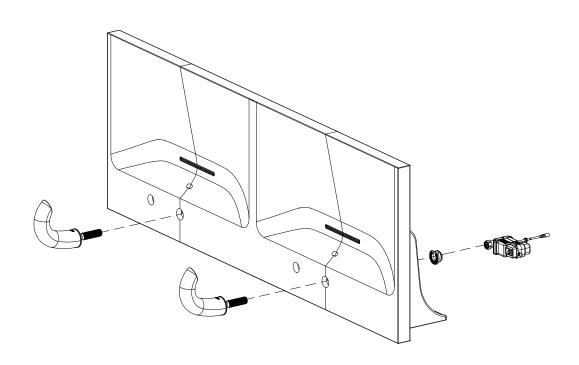
For ease of installion, lay basin on its back. Refer to faucet installation guide for details.
