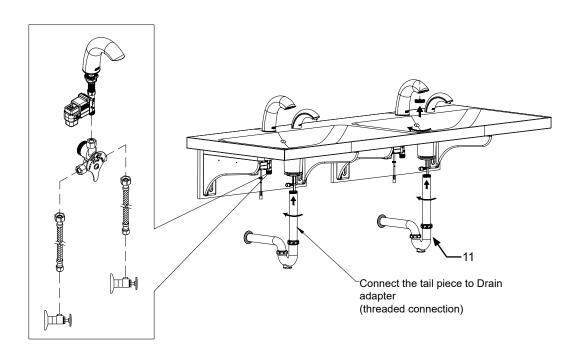
Adjust the tail piece base on drain outlet on the wall.
