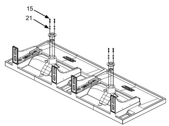
For ease of installion, lay basin on its top surface on a cushioned surface.
