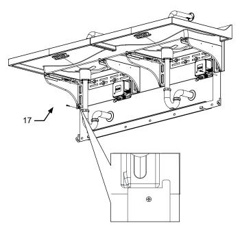
Align wall bracket as shown and install coarse screw on each side. Mark the slots in the wall bracket on the wall.
