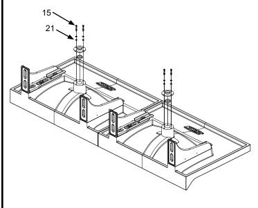
For ease of installation, lay basin on its top surface on a cushioned surface.
