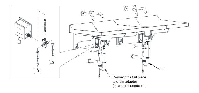
Adjust the tail piece base on drain outlet on the wall.
