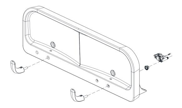
For ease of installion, lay basin on its back. Refer to faucet installation guide for details.
