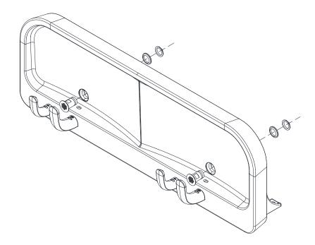
For ease of installion, lay basin on its back. Place grid drain into drainage opening Fasten washer and nut from underside of basin
