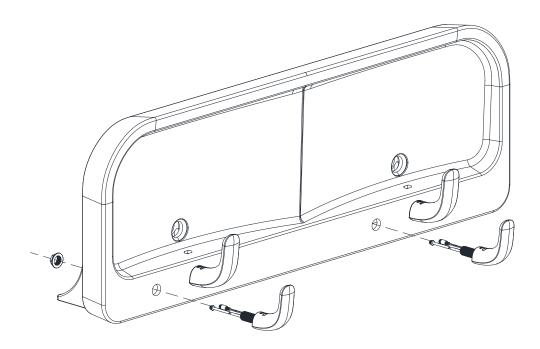
For ease of installion, lay basin on its back. Install the soap spout on right or left soap hole as applicable. Refer to soap dispenser installation guide for details.
