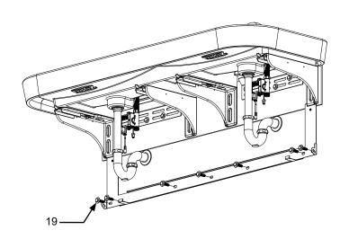
Re-install wall bracket with coarse screws in previous location. Then, fasten the wall bracket with 3/8" bolts through each holes and into the toggle bolts.
