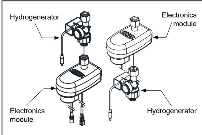
2. Connect electronics module power cable to hydrogenerator.
