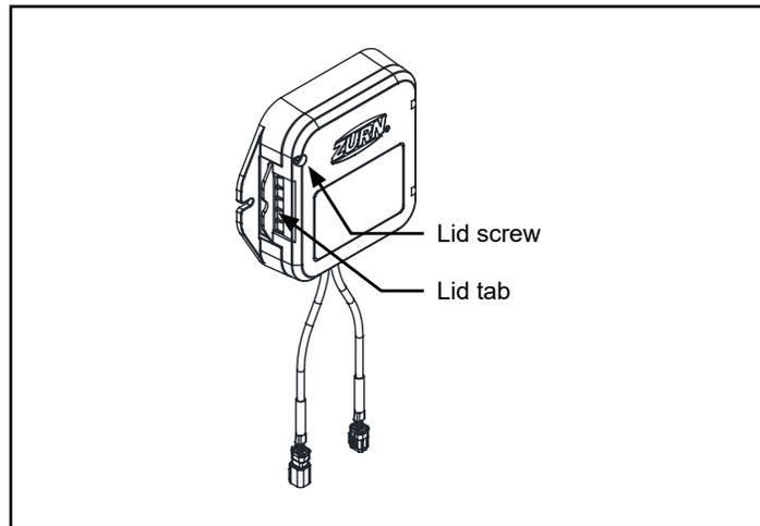
3. Install supplied alkaline batteries. Close lid and secure by pressing on the lid tab until it snaps into place. Then tighten lid screw.
