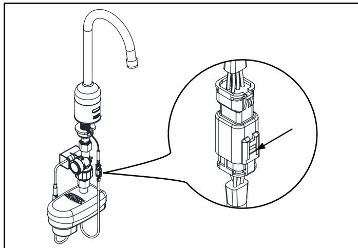
5. Connect the electronics module to the connected monitor first, and the spout to the connected monitor second.
