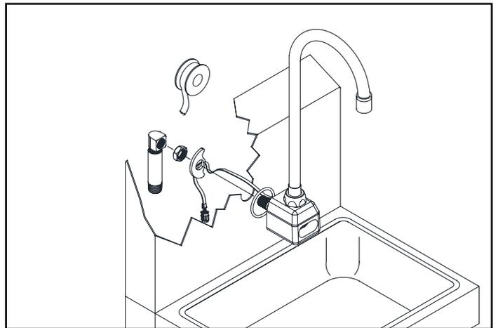
2. Ensure that slot in plastic washer is facing forward for Z6920, or facing downward for ZG6922 and sensor cable is routed outside of the plastic washer for both series.
