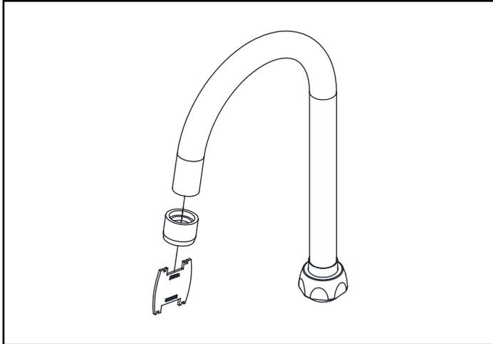
2. Install the spout onto the faucet body by turning the spout nut with an adjustable wrench clockwise.
