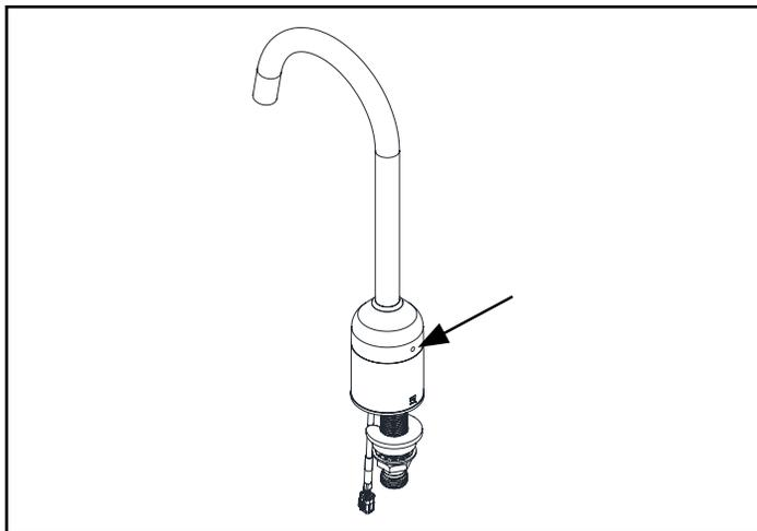
4. Carefully screw aerator into spout using the included tool.
