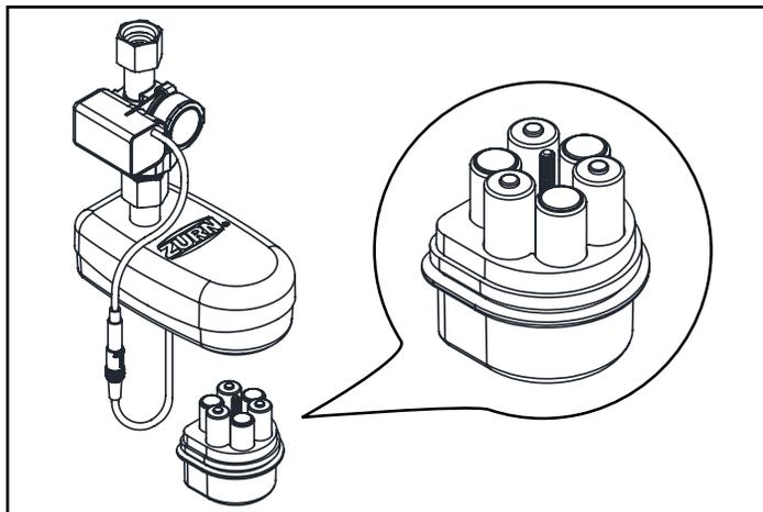
4. Tighten electronics module assembly with hydrogenerator to shank and connect water line(s).
