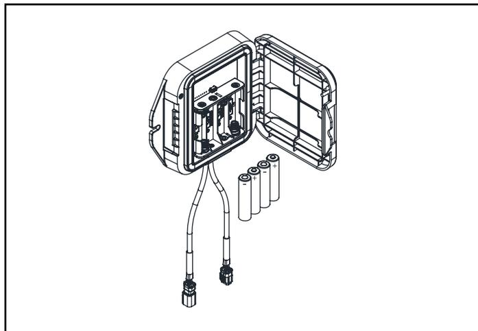
4. Unplug the sensor connection from the spout to the electronics module by compressing the clip on the connector and pulling apart.
