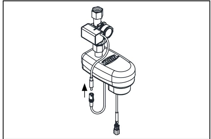
3. Open battery module using supplied hex key wrench and install supplied alkaline batteries in the electronics module in the configuration as shown.
