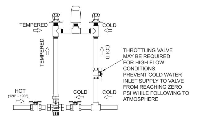
TYPICAL HORIZONTAL FEED FOR INSTALLATIONS WHERE TEMPERED OUTLET IS HORIZONTAL IT IS RECOMMENDED TO PLUMB THE HOT WATER FEED FROM ABOVE THE VALVE TO INSURE PROPER THERMOSTATIC OPERATION.
