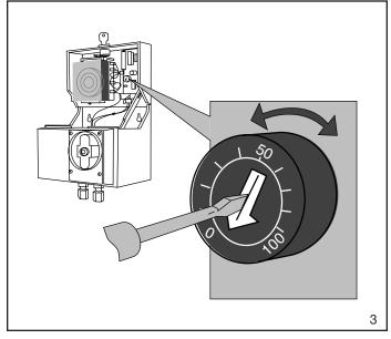
**3** To set the desired run time (dial setting): On the circuit board there is a small dial marked "0" to "100." These numbers do not represent time. This can be adjusted by turning the dial with a small screwdriver clockwise to increase time and counterclockwise to decrease time. Check pump run time with a watch to ensure proper dosage.
