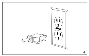
4 Plug pump into wall outlet. A GFCI receptacle is recommended. If the cord is not long enough, use a grounded extension cord at least 18 AWG. As with any electrical work, check your local codes first.
