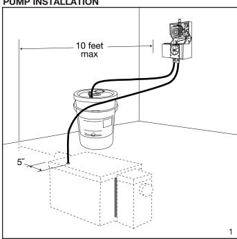
**1** Select a dry location to mount the pump. Attach the unit to the wall as close as possible to the Z1174 bacteria container and the interceptor. Supply tubing should not exceed 10 feet to or from the pump. \*Retrofit Kit (-RK) Installation: Drill a 7/16" hole in the interceptor cover five inches from the inlet side of the interceptor. It is very important to center the hole between scorations on the surface of the interceptor cover.
