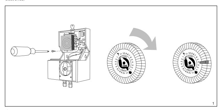
1 To set the current time, rotate the dial **clockwise** to the correct time. To select an "ON" time, lift the orange tab next to the time that you want the pump to turn on. An "UP" tab indicates that the pump turns on. A "DOWN" tab indicates that the pump will turn off. The Z1174 bacteria should be introduced into the interceptor after the kitchen is closed for the evening when little or no water is flowing through the interceptor. A one-half hour "ON" time should be adequate.
