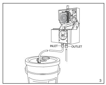
**3** Attach draw hose to inlet side of pump. Attach the supply hose to the outlet side of the pump. Make sure the compression fittings have the stainless steel ring and the ferrule installed correctly. Insert hoses into fittings completely and hand tighten. The supply tube should be inserted into the Z1174 bacteria bucket through the small access cap until it touches the bottom.
