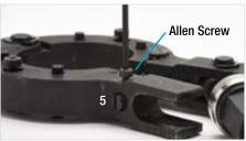
If necessary, remove existing jaw stop screw (#5), from the tool, by using an Allen wrench to first loosen the Allen screw, that holds the jaw stop screw in place, two rotations counter clockwise. Using a slotted screw driver, remove the jaw stop screw from the tool by turning it counter clockwise.
