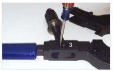
If necessary, remove existing E-Clip (#3) by prying it away from the pin with a flat head screw driver.
