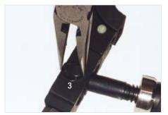
To install a new E-Clip (#3), place the E-Clip (#3) on the surface of the tool with it's opening positioned around the groove of the pin. Use needle nose pliers to push the E-Clip (#3) onto the pin until it snaps into place. (Note: The E-Clip will rotate freely but should not come off without prying with force.) Follow same procedure for E-Clip #2 (see above diagram for E-Clip #2 location).
