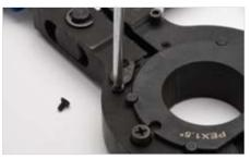
1. To replace the batteries, (that power the LED light), use a Phillips head screwdriver to remove the two screws that hold down the cover by rotating them counter clockwise.
