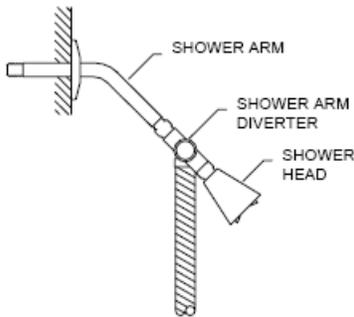
Thread swivel connection on to your present shower arm. Be sure all gaskets are in place. Attach shower head onto end of diverter in-line with shower arm. Attach hose to fitting 90° from center-line of shower head. Tighten all fittings and your shower is ready to use.
