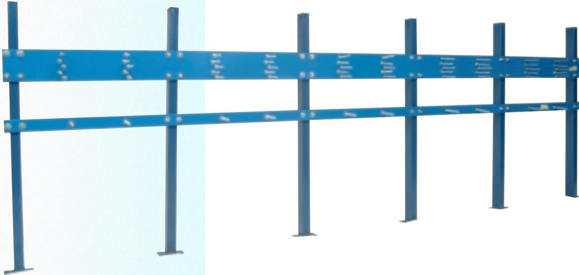
Multiple station plate system provides an extended length plate fabricated with exact center-to-center locations to accommodate a bank of multiple urinals. Custom-length plates are specific to job requirements and are provided with loose uprights and boxed mounting hardware and studs. Ideally suited for pre-fabricated applications.
