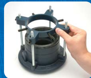
Thread rods into body and hand tighten screws.
