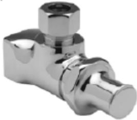
**Engineering Specification: Zurn Z81005-XL-LR-PC TO Z81017-XL-LR** - Polished chrome-plated cast brass angle stop fitting with ceramic disk cartridge, a loose key handle, one 12"[305mm] flexible chrome-plated copper lavatory riser complete with a wall escutcheon.
