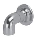
Engineering Specification: Zurn AquaSpec® Z80000-SE Bedpan washer flanged wall supply with a 1/2" female inlet and a 3/8" female outlet.
