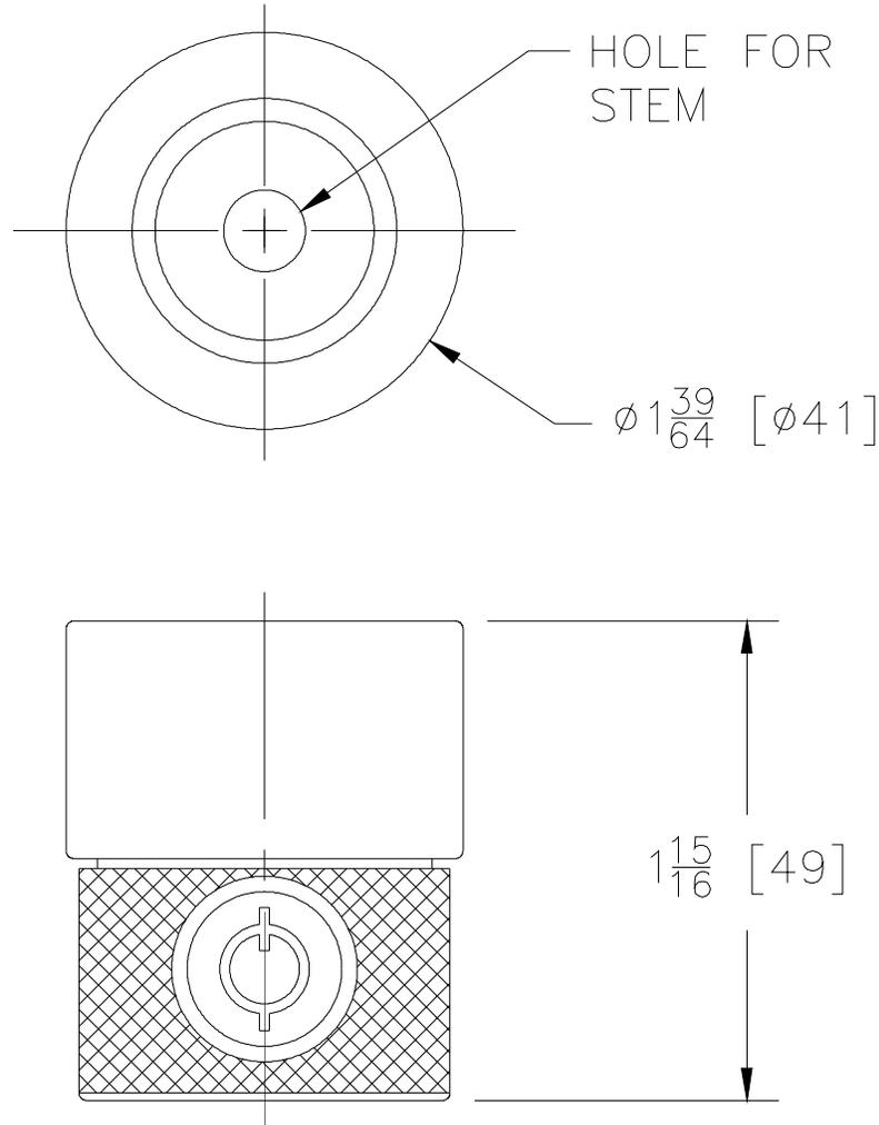
**ENGINEERING SPECIFICATION:** Z1399-HGS Brass hose bibb stem lock with key operated lock/un-lock feature.
