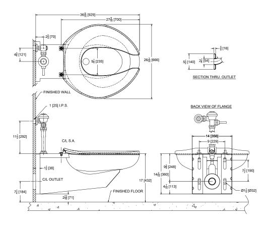
**Note:** For ADA compliance, rim height should be installed at 17"-19" from finished floor.
