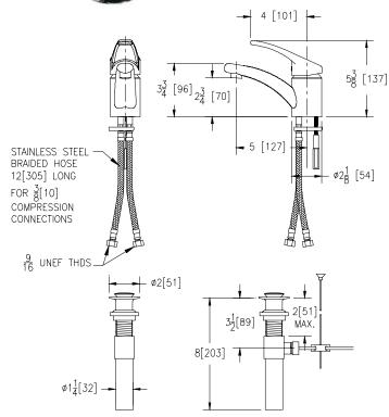
Zurn Lead Compliant\* "XL" products are a line of durable, high quality brass faucets and fixtures that are designed and manufactured to comply with state laws and local codes that mandate lead content levels. Zurn "XL" products are manufactured with \*not more than 0.25% lead content when used with respect to wetted surfaces of pipes and pipe fittings, plumbing fitting and fixtures: California Health & Safety Code § 116875; Vermont 9 VCA § 2470h
