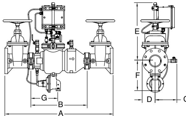
Attention: Model 375AW1 (grooved body) and Model 375W1 (flange body) have different lay lengths.
