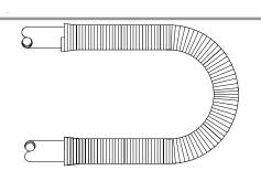
Step 4: Form the bend to the appropiate radius. A slight over bend initially helps the spring slide throughf after the final bend is formed.
