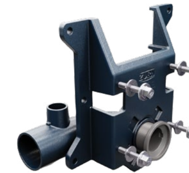
ZPWC1-NR4 ZPWC1 POD Pro Stud Supported Water Closet Carrier with 4" No-Hub Right Hand Horizontal Cast Iron Fitting
