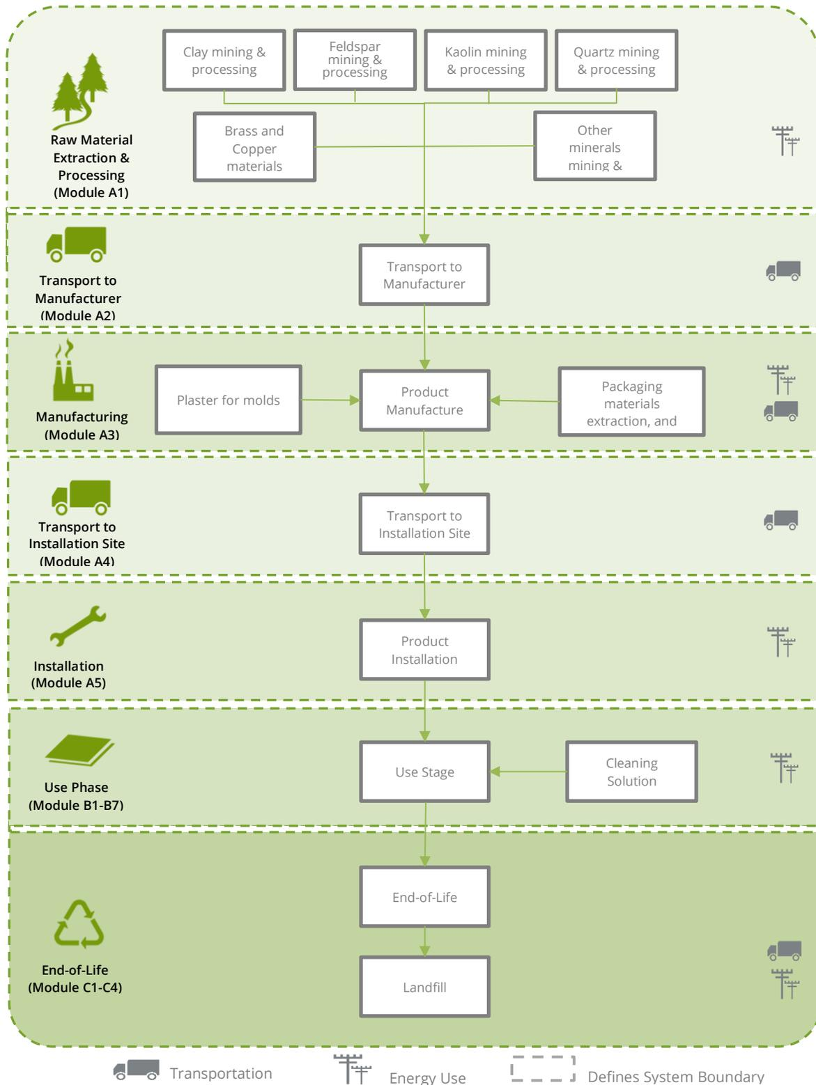
Figure 1. Flow diagram for the Zurn vitreous china urinals.
